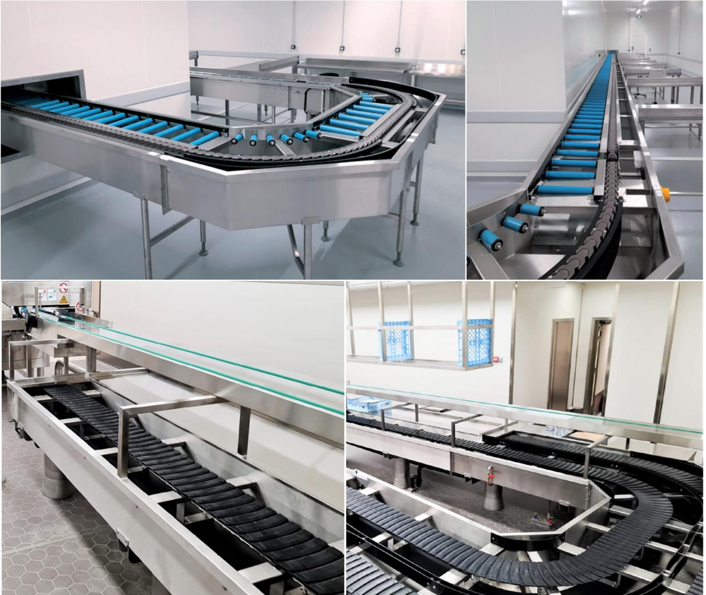
Our customized bi-cord transport system is the perfect solution not only to carry, but also to wash and deliver trays. The system limits the workers operations and contains management costs and space while perfectly drying the trays for an immediate use.
