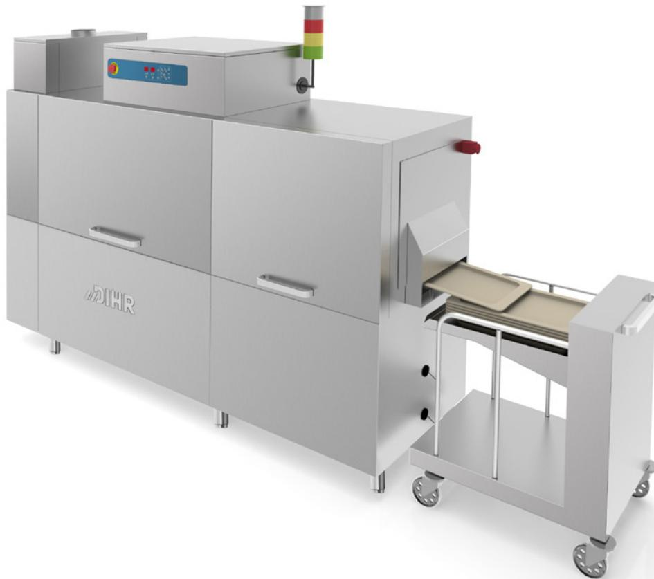
The standard heat recovery uses the steam produced by the machine to preheat the incoming cold water for immediate energy savings. The special twin-cord conveyor system, sloped and separated by zone, avoids any contamination
